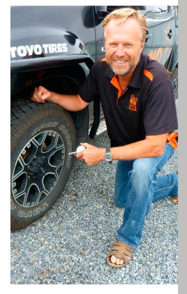
simply, don't be afraid to let a lot of air out if the surface demands it. Let's start with a well-made dirt road with typical corrugations on the corners, a loose surface of gravels and maybe pockmarked with the odd pothole. At full road pressures (refer to your placard) your tyres will be working pretty hard to keep delivering the required grip, great on the bitumen, horrible on anything else. If you've noticed that on those same bends your vehicle is doing
